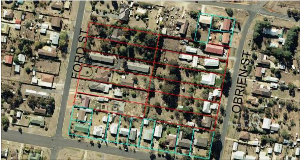
Figure 3.3 Orthogonal grid subdivision typology
