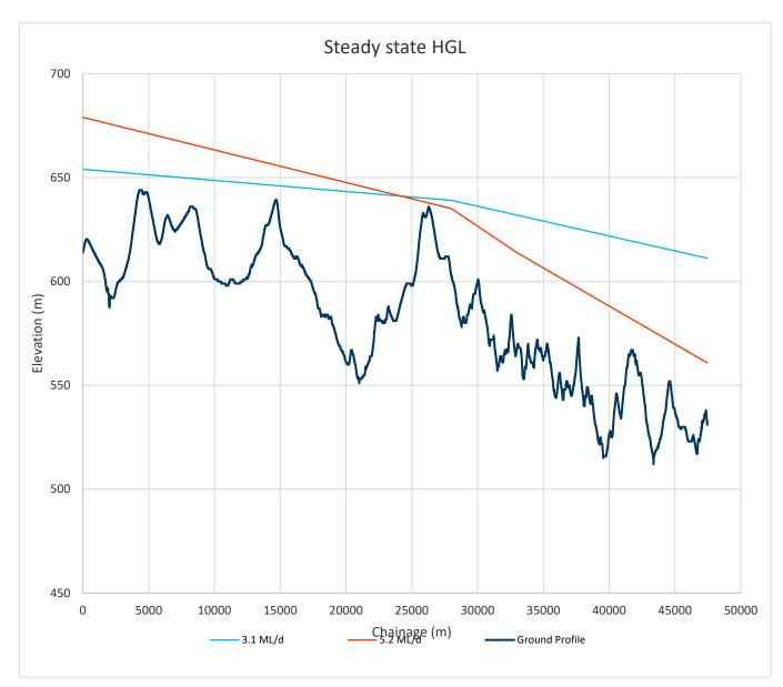
Figure 7-3 Hydraulic Grade Lines – gravity option
