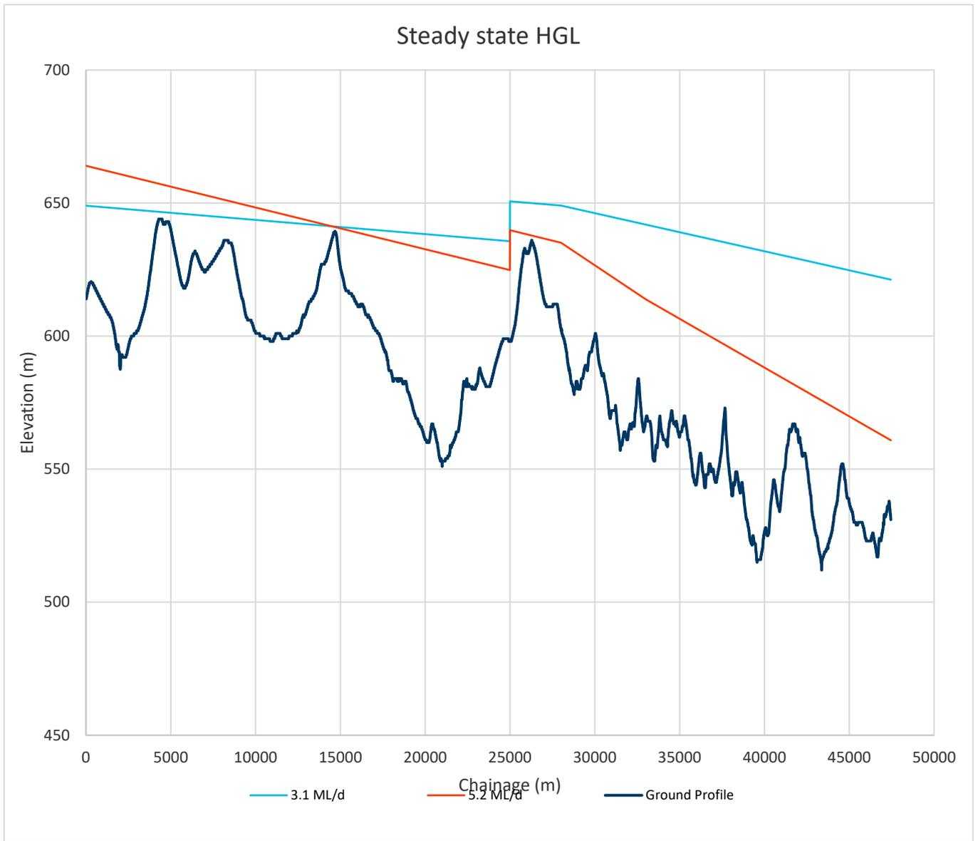
**Figure 7-4** Hydraulic Grade Lines with pump station
